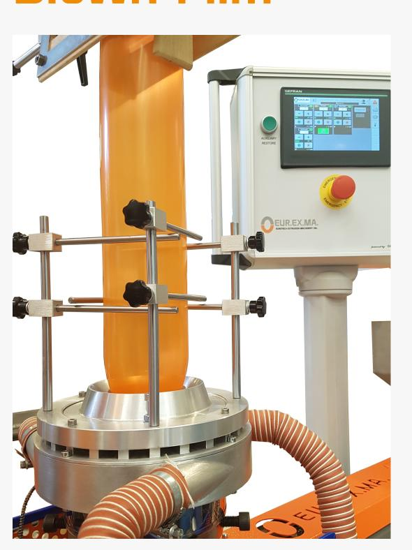
Blown Film Lines are used for the extrusion of mono-layer or multi-layer tubular film, that can be used to test polymers (virgin, recycled or biopolymers), in order to perform quality tests and produce samples for packaging and medical applications.
