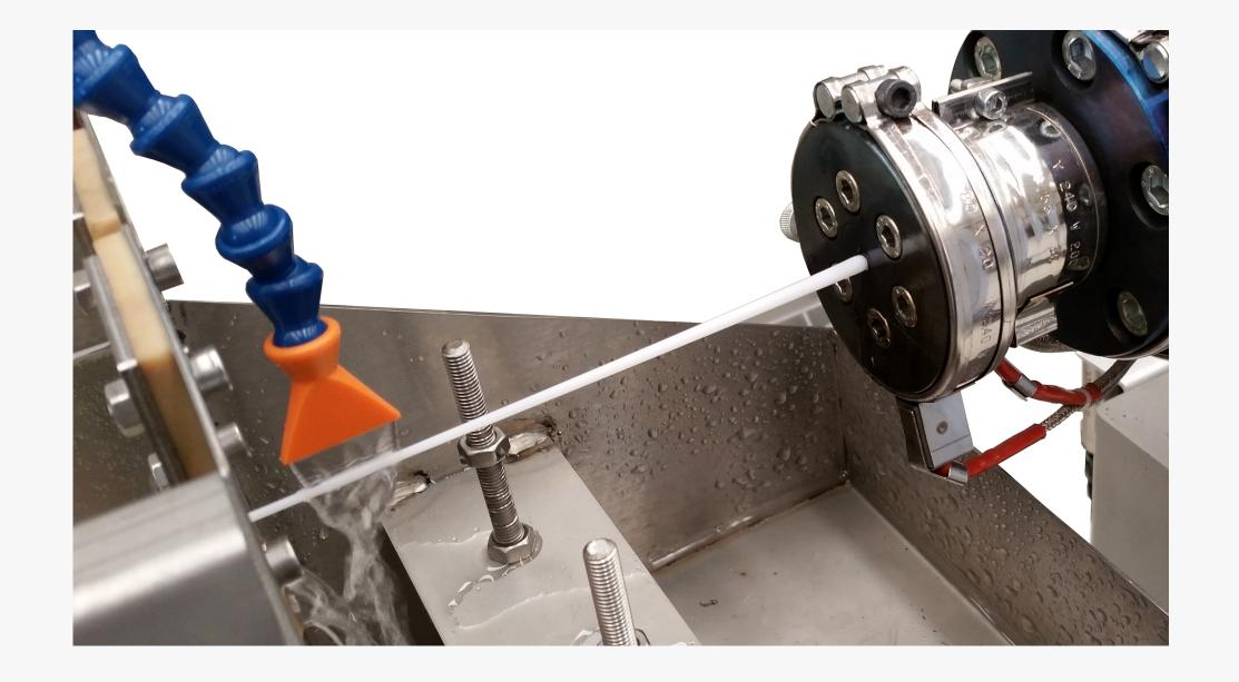
3D filament lines are used for the production of filament for 3D printing. They can process standard materials such as ABS, PLA, PE, TPU or, if equipped with a double cooling system (air/water), also several kinds of technopolymers.
