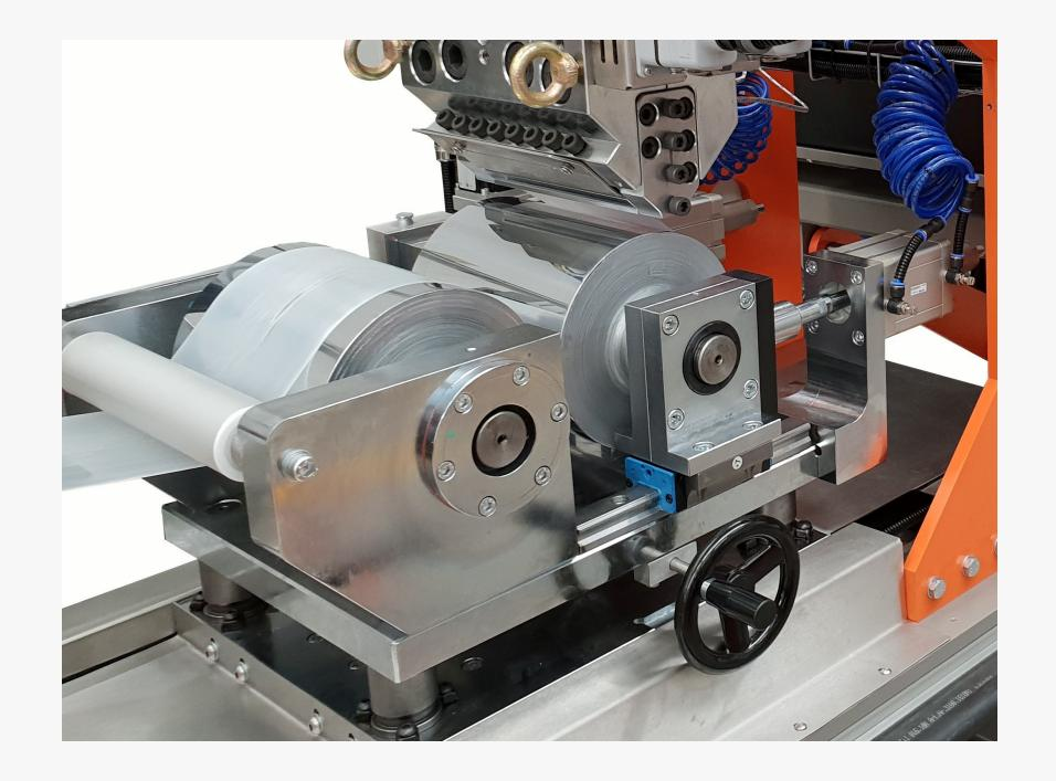
Cast film lines are designed for the production of samples of film for quality testing with a wide variety of polymers, from standard polyolefines to biopolymers and technopolymers, with a thickness range from 20 to 1000 microns.
