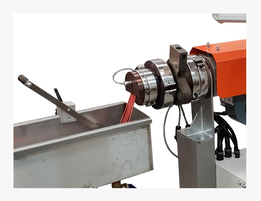
Compounding lines are used to produce granules of polymeric materials, virgin or recycled. They can be composed of single-screw extruders or co-rotating twin-screw extruders, used to test different formulations of masterbatch and compound, including plants for biodegradable resins.
