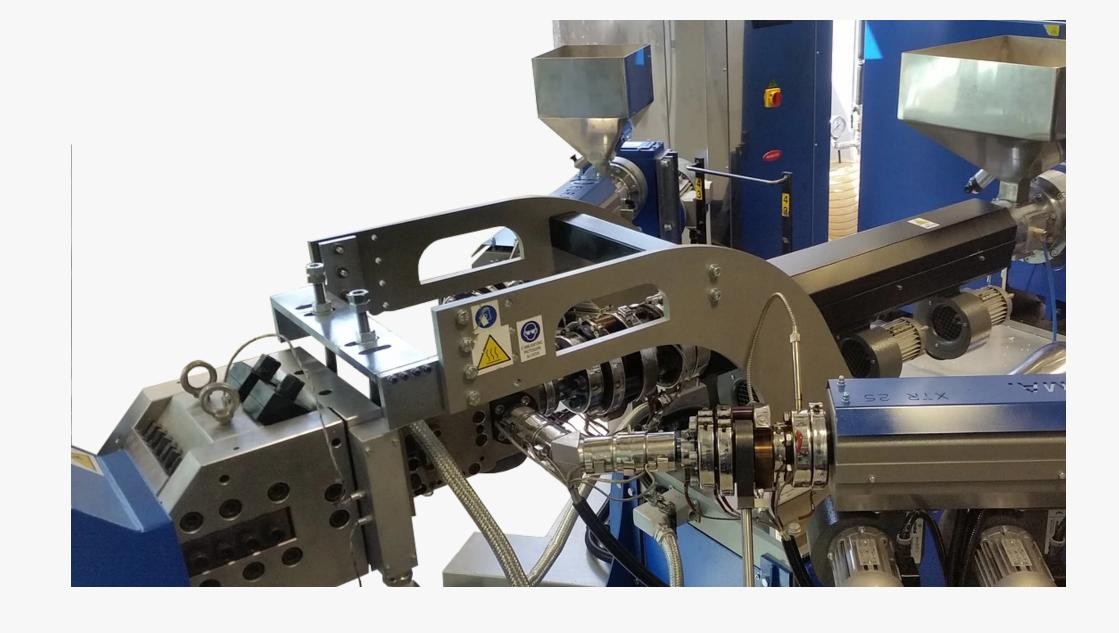
Foil lines are designed for the extrusion of mono-layer or multilayer foil samples from 1 to 10 mm of thickness, with a wide variety of materials. They can be equipped with winders for reels or guillotine cutting units for sheets.
