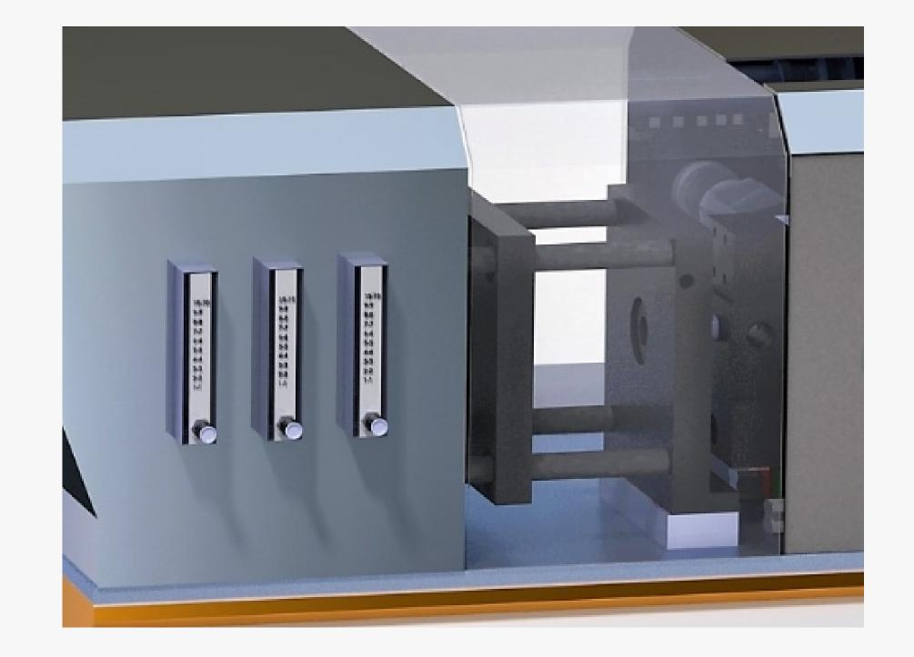
Our injection moulding laboratory line is useful to test every kinds of polymeric materials. With this line, it is possible to create samples with a very low amount of material in order to perform quality tests before starting with the serial production.
