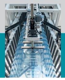
5-layer co-extrusion Blown Film R&D line
