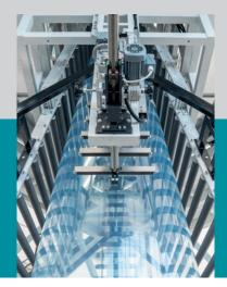
3-layer co-extrusion Blown Film R&D line
